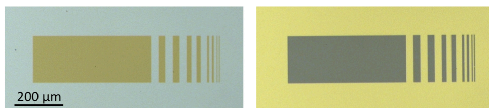
Figure 1: optical microscopy images of a section of the surface of samples for XPS calibration. Left: Au patterns in Ag; right: Ti patterns in Au. The grating of stripes is dedicated to the determination of lateral resolution.
