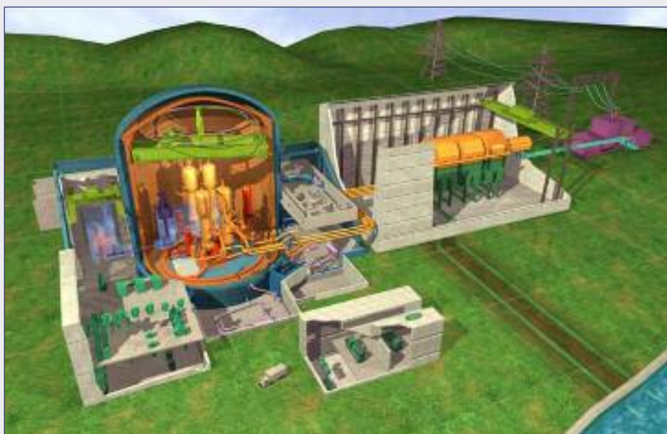
Fig. 2 - Schematics of EPR, with turbine building and water cooling. No big hyperboloid cooling towers and scrubbers are necessary for the operation, but just a vast source of cooling water
