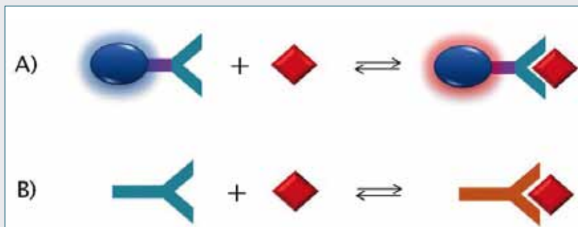
Fig. 1 - Schematic representation of A) a luminescent sensor and B) a colorimetric sensor
