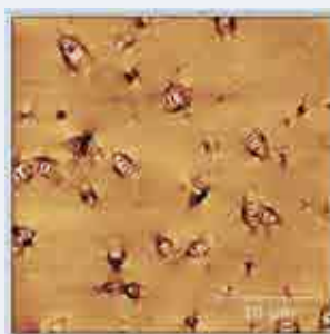
Fig. 3 AFM analysis of bitumen showing micelles made of asphaltene core (bees) with a shell of highly polar resins
