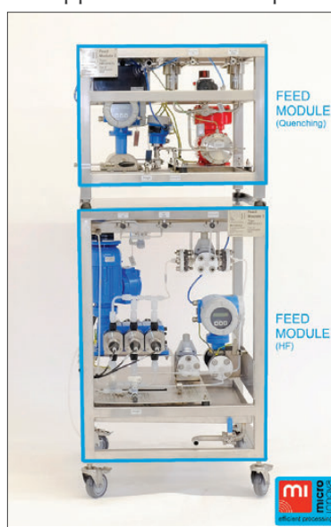
Fig. 4 - Example of two modules for API production
