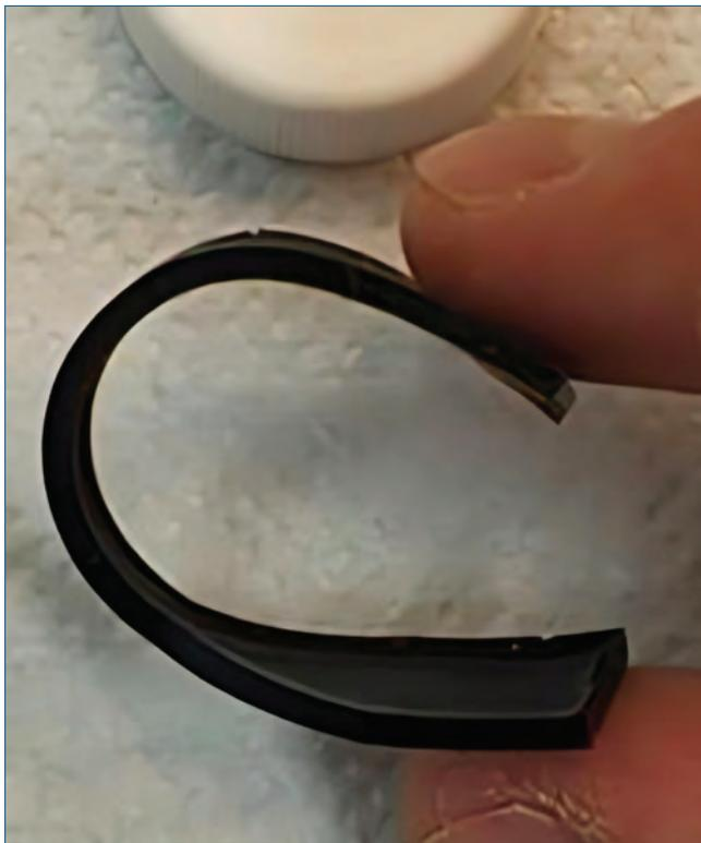
Fig. 1 - Prototype of lignin-based epoxy resin
