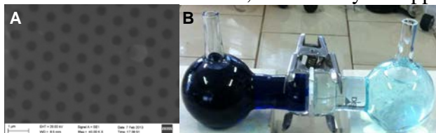
Fig. 1. A) SEM image of silica porous film deposited on \text{Si}_3\text{N}_4 macrosieves. B) Microfluidic device.
