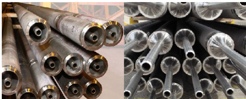
Fig. 10 - Tubi di reforming (Manoir Industries)
