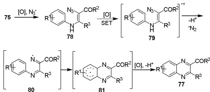
**Scheme 34.** Cascade reactions of enamine and  $\text{TMSN}_3$  for quinoxaline synthesis.
