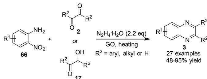
**Scheme 31.** Synthesis of quinoxalines using *o*-nitroanilines and vicinal diketones via hydrazine reduction.
