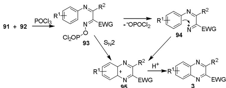
**Scheme 36.** Cascade reactions of anilines and  $\beta$ -keto oximes for quinoxaline synthesis.
