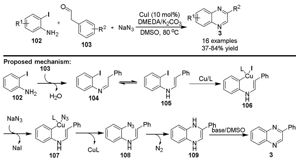
**Scheme 39.** Copper-catalyzed cross-coupling cascade synthesis of quinoxalines.
