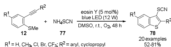
Scheme 38. Synthesis of 3-thiocyanatobenzo[ b ]thiophenes 78 under photocatalyzed reaction.
