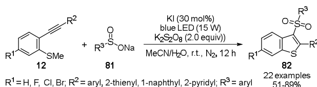
Scheme 40. Visible-light-mediated synthesis of 3-sulfonylbenzo[ b ]thiophenes 82 .
