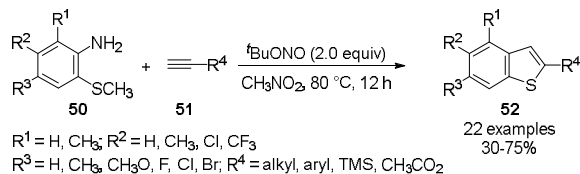
Scheme 24. Synthesis of 52 from 2(thio)arylamines and terminal alkynes.
