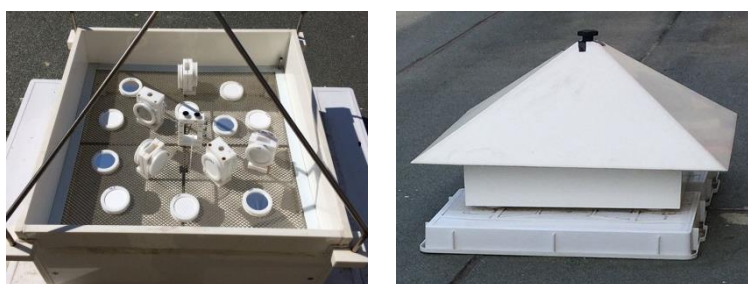
Fig.1: The inner and the external features of Deposition Box during the exposures of surrogate surfaces.
