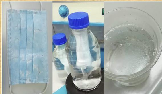
**Fig. 1.** Pictures from the experimental procedure. From the left to the right: (a) a surgical mask after prolonged UV light exposition (b) surgical mask stirred inside a bottle filled with artificial seawater solution (c) appearance of the microfibers “soup” on the top of the artificial seawater solution at the end of the artificial weathering treatment.
