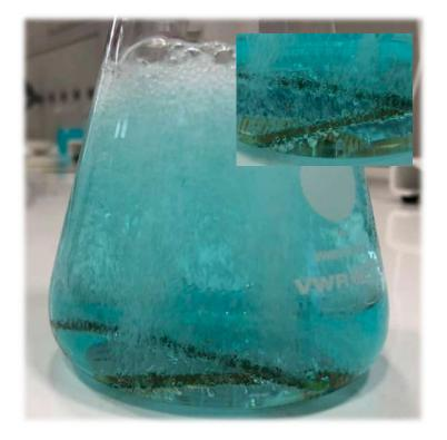
RT: energy saving and safe process  $H_2O_2+2H^++2e^- \rightarrow 2H_2O$  $Cu \rightarrow Cu^{++}+2e^-$
