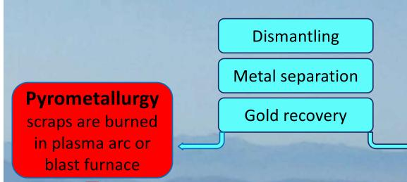
Floating slags, sinking sludges, oils from plastics, solid waste and toxic emissions are produced (at 1250 C lead vapors, dioxins, and furans are released)
