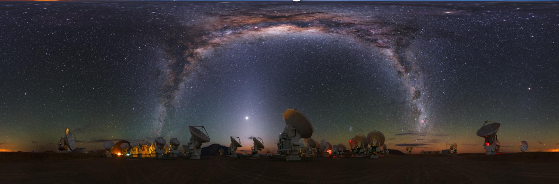
ALMA (Atacama Large Millimeter/submillimeter Array): 66 antennas - range: 84-950 GHz
